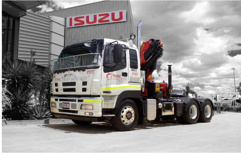
Prime Mover Crane Truck Front Fitted -- PK 18002D Palfinger Crane -- Max 5, 750kgs (See Below)
