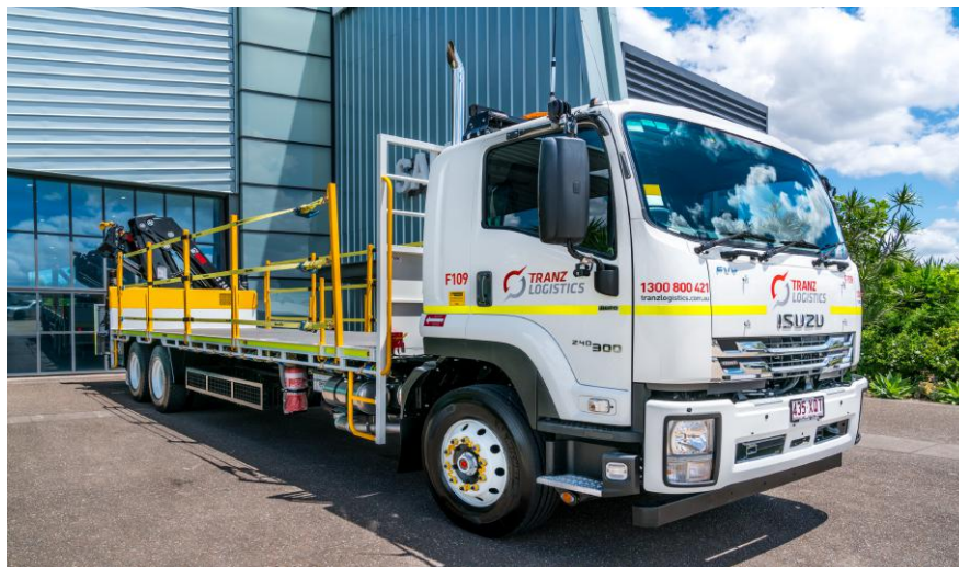
Flatdeck Crane Truck with 9m Tray Front Fitted - HIAB XS 288 EP4 Crane -- Max 9, 500kgs (See Below)
