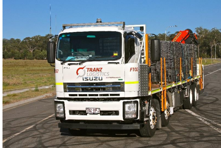
¾ Cab Flatdeck Crane Truck with 12/9m Tray Rear Fitted - PKG 14002 Palfinger Crane – Max 6,1000kgs (See Below)
