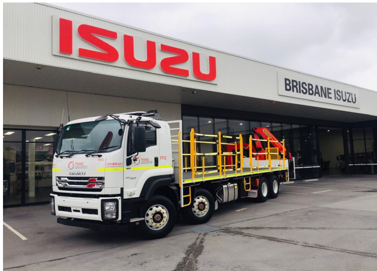
Flatdeck Crane Truck with 9m Tray Front Fitted - PK 26002 EH Palfinger Crane -- Max 8, 500kgs (See Below)
