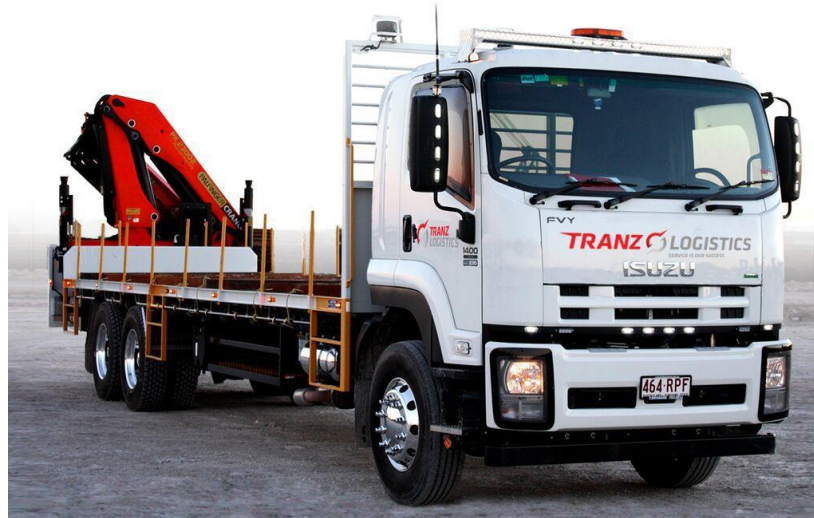
Flatdeck Crane Truck with 9m Tray Front Fitted - PK 14002 EH Palfinger Crane – Max 6,100kgs (See Below)
