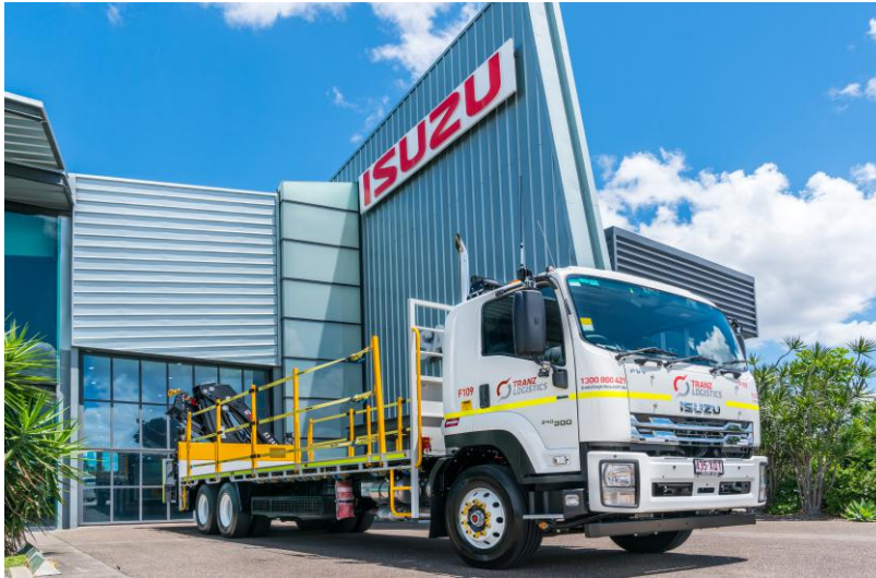
Flatdeck Crane Truck with 9m Tray Front Fitted - HIAB XS 244 EP4 Crane -- Max 9, 500kgs (See Below)
