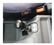
Park Brake Alarm – Activates horn if door is opened and park brake not engaged.
