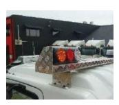
Mine Spec - Roof Mounted - Indicator, Brake and reversing lights
